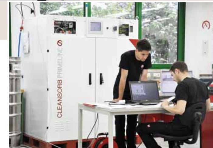
When configured for hydride gas processes such as MOCVD, unique control functions include an infra-red array for contactless temperature monitoring of the absorber columns, as well as an inert gas cooling mechanism. A dedicated class of CLEANSORB chemisorber media ensures highly effective, temperature-managed removal of toxics such as arsine or phosphine.
